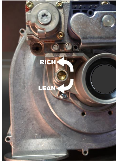
Illustration 2 - Air/Gas Mixture Ratio Screw
